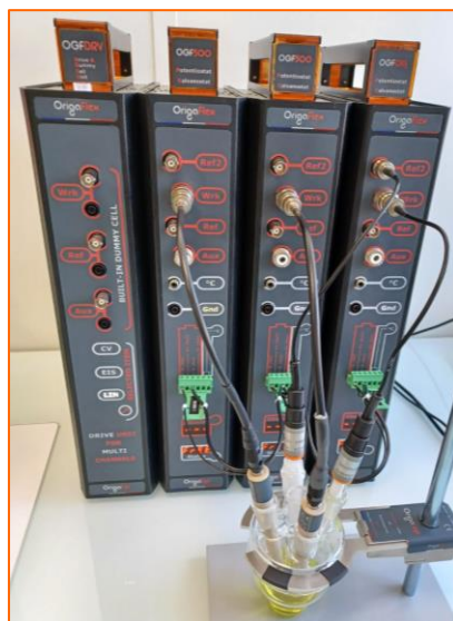
Figure 6: Bipotentiostat manipulation on Ferri/Ferro Cyanide couple
