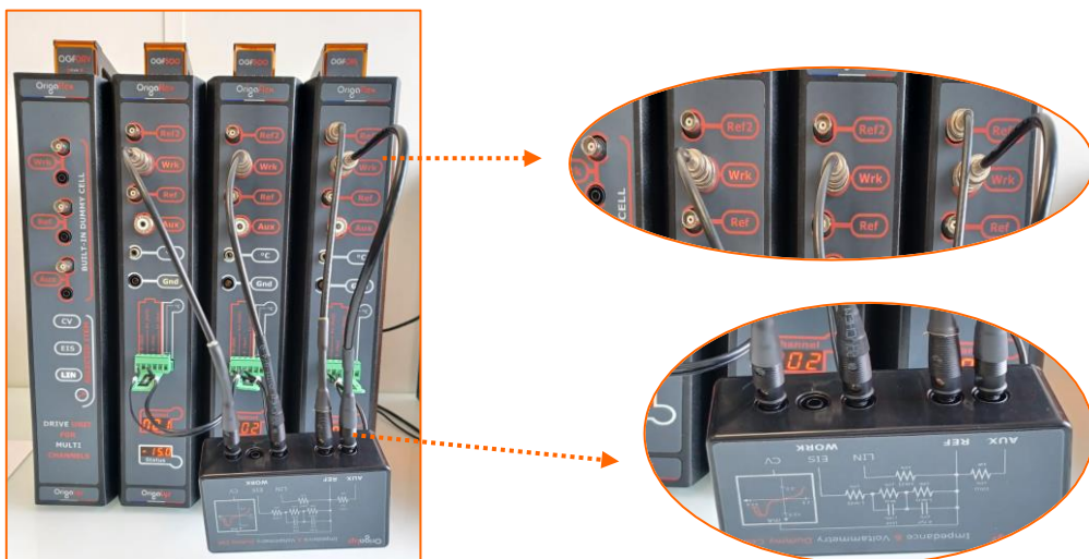
Figure 2: Connecting Dummy Cell to Bipotentiostat
