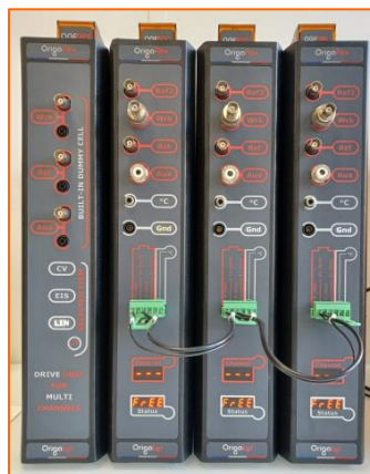
Figure 1: scheme (a) and real (b) configuration of bipotentiostat
