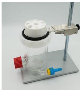
Figure 14: Electrochemical cell
