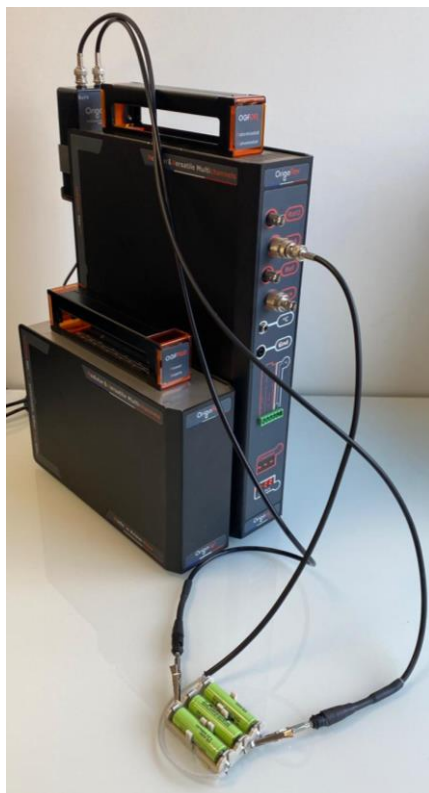
Figure 1: Battery samples connected to potentiostat.
