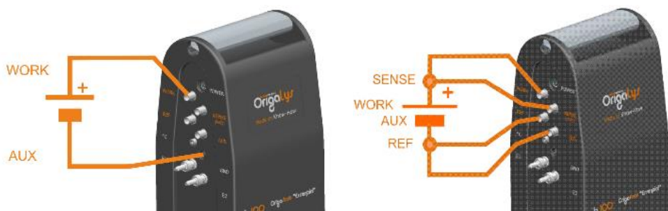
Figure 1: The left photo shows 2 electrode configuration and the right photo is about 4 electrode configurations with a potentiostat
