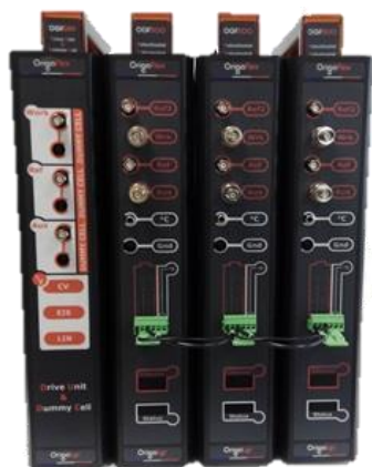
Figure 8: Multi Potentiostat, all tests of this application note were performed on second channel
