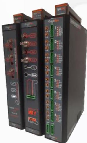
**Figure 1: OrigaMux module connected to OrigaFlex potentiostat**
