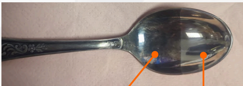
Figure 7: Spoon after restoration by electropolishing
